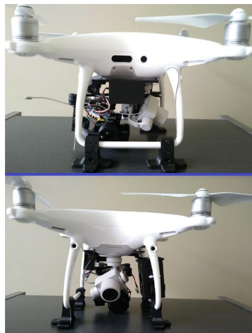
Fig. 7. Drone with RGB and thermal camera used in this work.
